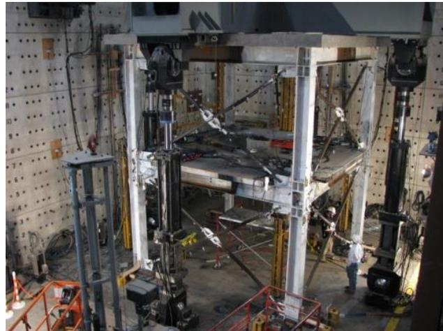
**Figure 4:** Two-story steel braced frame test
