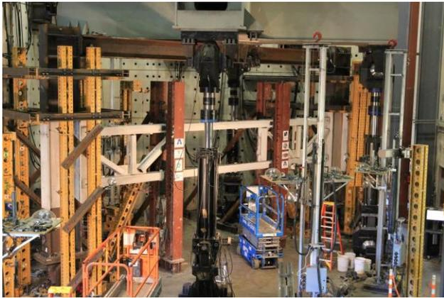
**Figure 3:** Special truss moment frame (STMF) test
